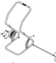
2 Insert the axle (13) into the openings on both sides of the frame (2). Slide the solid wheels (14) over the axle and make sure the wheel caps are facing outwards. Secure the wheels onto the axle with Ø10 washers and M10 nylon nuts (19) using a spanner.
