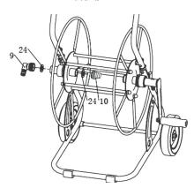
**6** Mount the  $\frac{1}{2}$ " (13 mm) male inlet swivel valve (9), with the rubber washer (24) in between, onto the flange end and tighten by hand or with the aid of a tool. Place the  $\frac{1}{2}$ " (13 mm) male outlet hose coupling (10), with the rubber washer (24) in between, onto the outlet hose coupling of the reel. Tighten by hand or with the aid of a tool.
