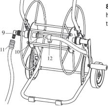
**8** Attach the long hose via the  $\frac{3}{4}$ " male outlet hose coupling (10) onto the reel and secure with the hose clamp (12).
