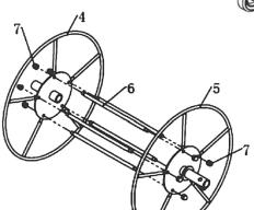
**3** Insert the two ends of the connecting rods (6) into the openings provided for this purpose in the right-hand (4) and left-hand (5) flanges. Fasten using an M8 cap nut (7).
