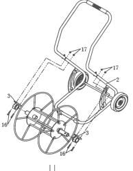
**4** Mount the two bearings (3) in the ends of the flanges (4 & 5). Align the bearing openings (3) with the openings in the frame (2). Secure both sides of the bearings with an M6 x 30 bolt (16) and an M6 nylon nut (17) using a spanner and the Allen key supplied.
