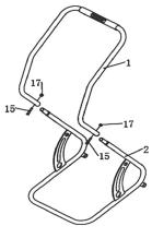
**1** Slide the U-handle (1) onto the frame (2). Insert an M6 x 25 bolt (15) into one of the holes in the frame and secure with an M6 nylon nut (17) using a spanner and the Allen key supplied. Do the same on the other side.
