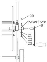
**5** Insert the crank handle (8) into the hub of the flange end (5). Align the openings in the hand crank and secure with an M8 x 40 bolt (20), M8 washer (21), M8 spring washer (22) and an M8 nylon nut (23) using a spanner and the Allen key supplied.
